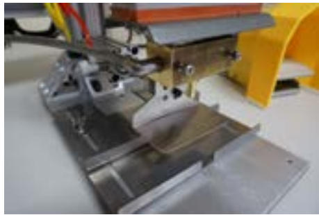
Model shown: RX-95-PS2-RK Single Hole Punch with basic controller (shown with optional Slug-Tray below)
