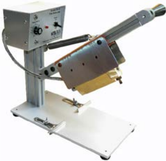
Model shown: RX-80-BHL-RK 4" (110mm) Brass Hot knife with interchangeable Punch Collet (see custom configurations on back)
