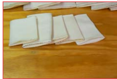
Cuts and seals without closing the ends
